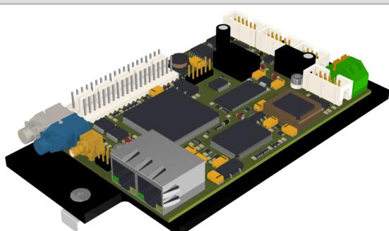
**SMM 400 Bus-Master** provides the interface between personal computer (via ETHERNET) and the system modules over RS 485-Ringbus.
