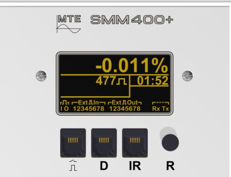
**SMM 400+** Meter Evaluation Module with large color display, Reset – button and 2 scanning head pulse inputs is the perfect solution to test modern meter. The sockets are used for:
